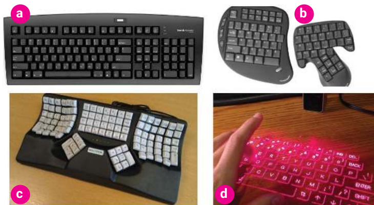
Gambar 4.5 Jenis-jenis keyboard. (a) Keyboard Dvorak, (b) Keyboard Klotenberg, (c) Keyboard Maltron, (d) Keyboard Virtual
